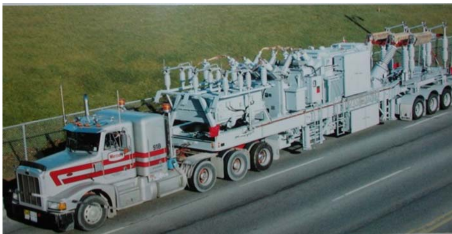
Figure 7. Mobile substation in transit.
