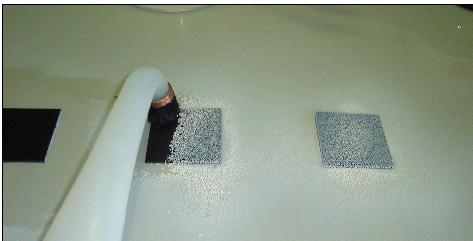
Figure 8. SX34 applied (white powder) on material and removal of residues.
